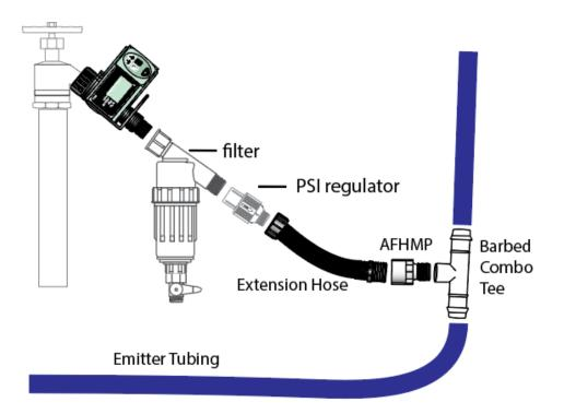
Once your emitter tubing is connected to the fitting, you will lay the tubing around the base of your home. The tubing should be placed a minimum of 12" away from the foundation, but within 18" for optimal foundation watering. Use the hold downs to keep the tubing in place. You can trench and bury the tubing up to 6" deep. Another option would be to mulch over the tubing to protect it from the elements or hide it from view.
